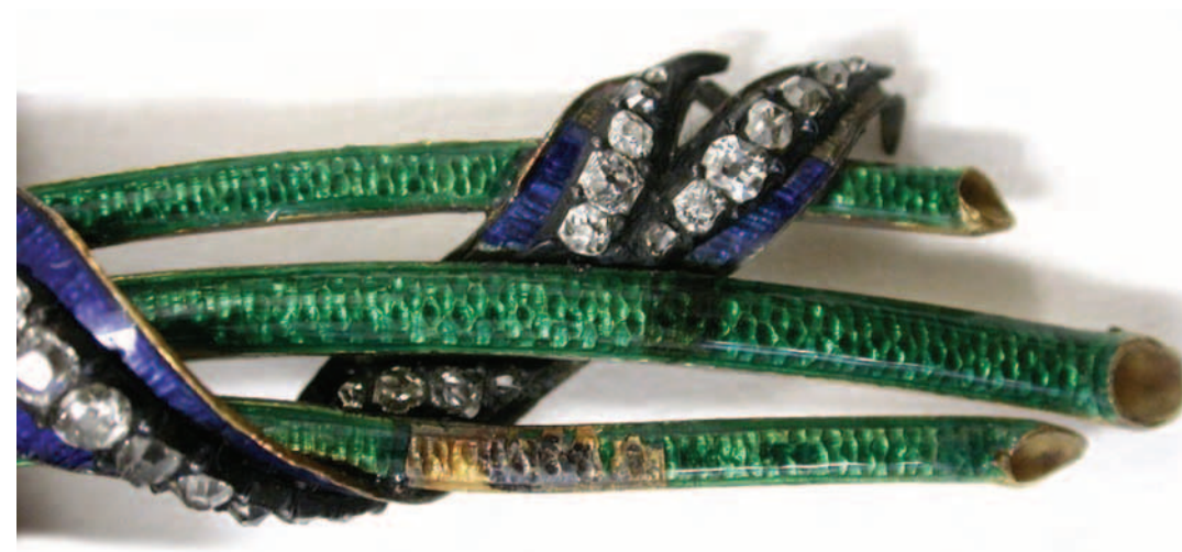
Figure 3. Lower section of bodice ornament showing the tarnished gold alloy and the loss of enamel.
